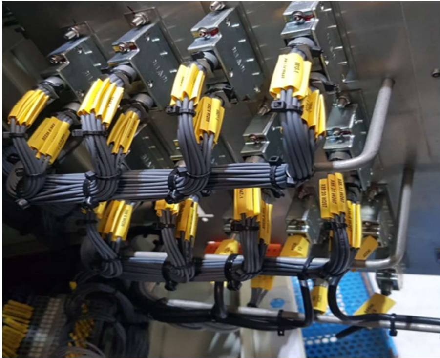
Assembly of ready to fit harness in panel
